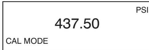
Use the Pressure Standard to output 437.50 psi (87.5%). After the output has stabilized, press the ENTER key to continue. As the unit takes readings, the screen will show \_\_\_\_\_. When the readings are complete the screen should look as shown below.
