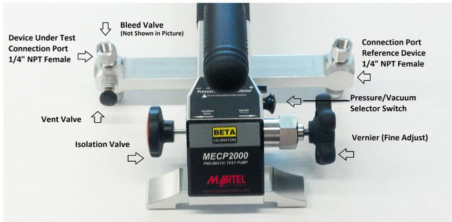
1. Inspect the fitting or device to be installed on the pump to be sure it is clean and the threads are in good condition. Clean or replace if necessary.
